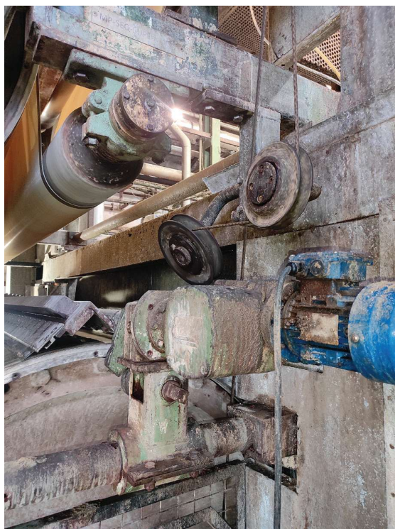
Figure 1: The outdated gravity-loaded rigid doctor with electromechanical oscillation that was replaced.
