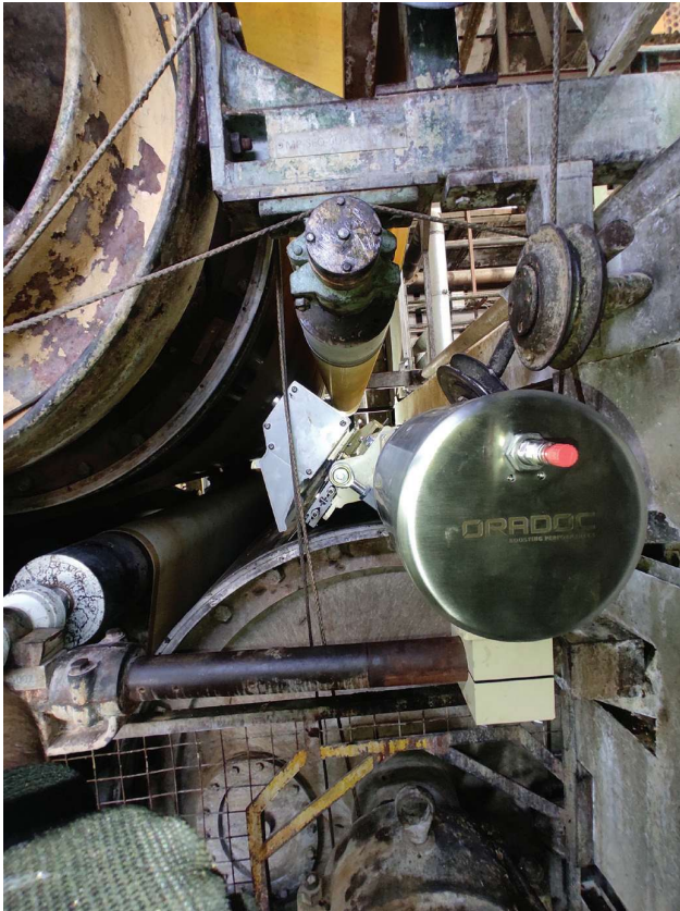
Figure 3: OraFlex doctoring system with pneumatic oscillator.
