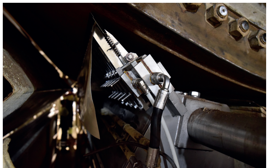
Figure 3. OraCrepe blade holder installed on Yankee roll.
